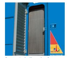
Separated oil cooler from engine radiator
