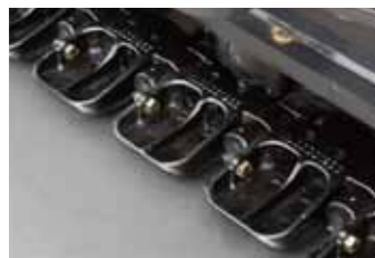
High-durability box type track shoes
